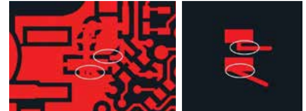
Areas that do not meet the permissible DRC parameters
